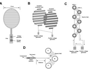
Fig 1 Diagram of the racket-shaped electrostatic flying insect catcher (REIC) (A), two layers of ICWs oppositely charged with two voltage generators (B), electric fields formed between ICW(-) and ICW(+) (C), and an insect blowing assay (D). The arrows show the direction of the flow of free electrons between ICW(-) and ICW(+) to form the electric field (C) and the direction of the path taken by the insects due to the electrostatic forces (D).
