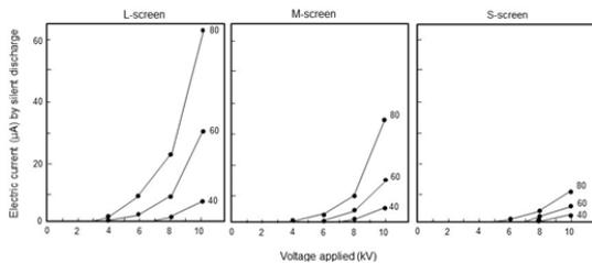
Figure 3. Relationship between the applied voltage and magnitude of current generated by the silent discharge from the central net (CN) of the three types of electrostatic window screen under different relative humidity (RH) conditions. The numbers in the figure represent RH (%).
