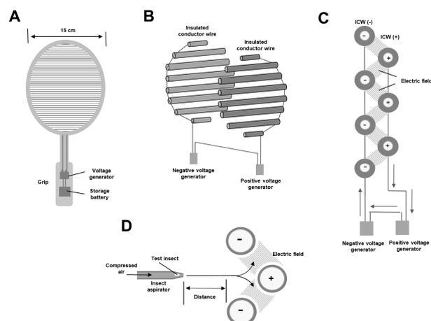
**Fig 1** Diagram of the racket-shaped electrostatic flying insect catcher (REIC) (A), two layers of ICWs oppositely charged with two voltage generators (B), electric fields formed between ICW(–) and ICW(+) (C), and an insect blowing assay (D). The arrows show the direction of the flow of free electrons between ICW(–) and ICW(+) to form the electric field (C) and the direction of the path taken by the insects due to the electrostatic forces (D).
