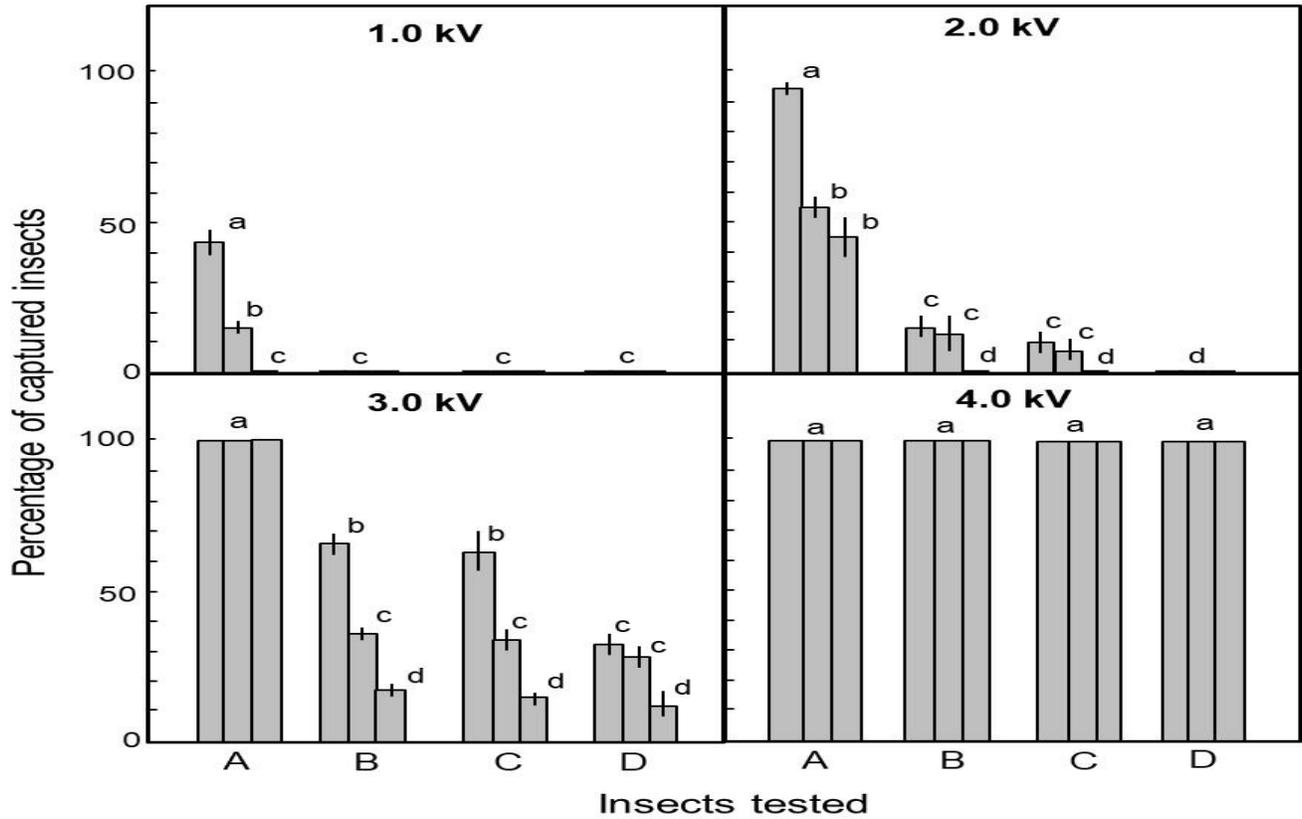
**Figure 3.** Insect pests captured with the ICWs of the electric field screen. The ICWs of the electric field screen were doubly charged with 4.0 kV, and adult whiteflies (A), western flower thrips (B), green peach aphids (C), and tomato leaf miner flies (D) were separately blown toward the ICWs at 3 m/sec.
