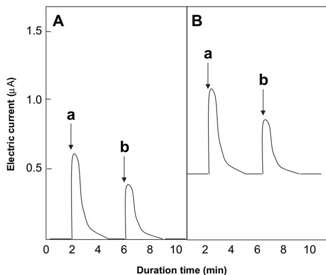
**Fig. 4.** Electric current generated at the time of insect-capture with the ICW at the lower voltage range (4.1-kV charge) (A) or at the higher voltage range (5.2-kV charge) (B). The arrows 'a' and 'b' represent the timing of blowing an adult vinegar fly or cigarette beetle, respectively, into the screen.
