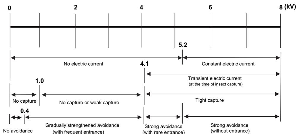
**Fig. 6.** Schematic expression of voltage ranges applied to the screen in terms of electric current generation, insect-capture capability, and induction of avoidance responses of adult cigarette beetles and vinegar flies.
