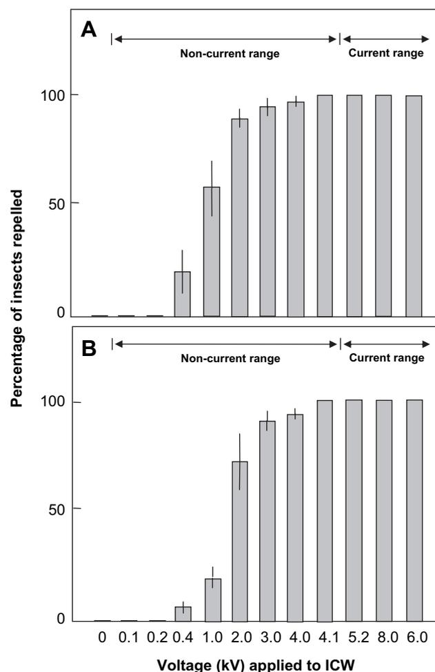
**Fig. 5.** Repellence of cigarette beetle (A) and vinegar fly adults (B) by the electric field screen placed in the middle of a transparent acrylic cylinder. After reaching the net of the screen, the insects passed through the screen (non-repelled) or removed themselves from the screen without entering (repelled). The data were given as means and standard deviation of five replications.
