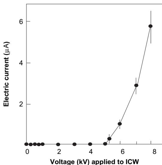
Fig. 3. Relationship between voltages applied to the ICW and the electric current flowing from the ICW to the earthed nets.
