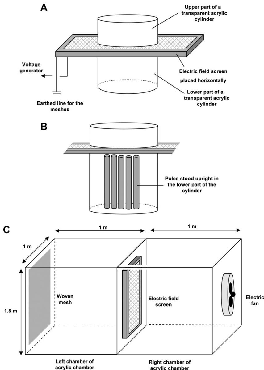
**Fig. 2.** Structures of the screen cylinder (A and B) and screen chamber (C) used in the present study. Poles were placed upright in the lower part of the screen cylinder to use a climbing assay of cigarette beetle adults released at the bottom.
