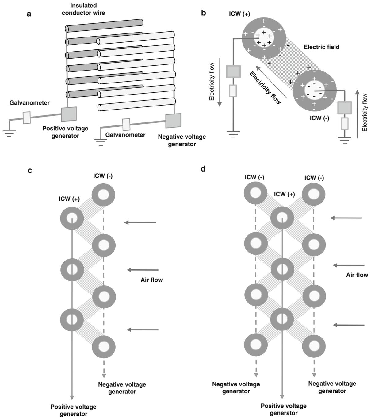
**Fig. 1** Diagram of components (**a**) and cross-sectional views of insulated conductor wires (ICWs) (**b–d**) in the electric field screens. **a** Layers of ICWs arrayed in parallel and linked to each other and grounded DC voltage generators. **b** The electric field
