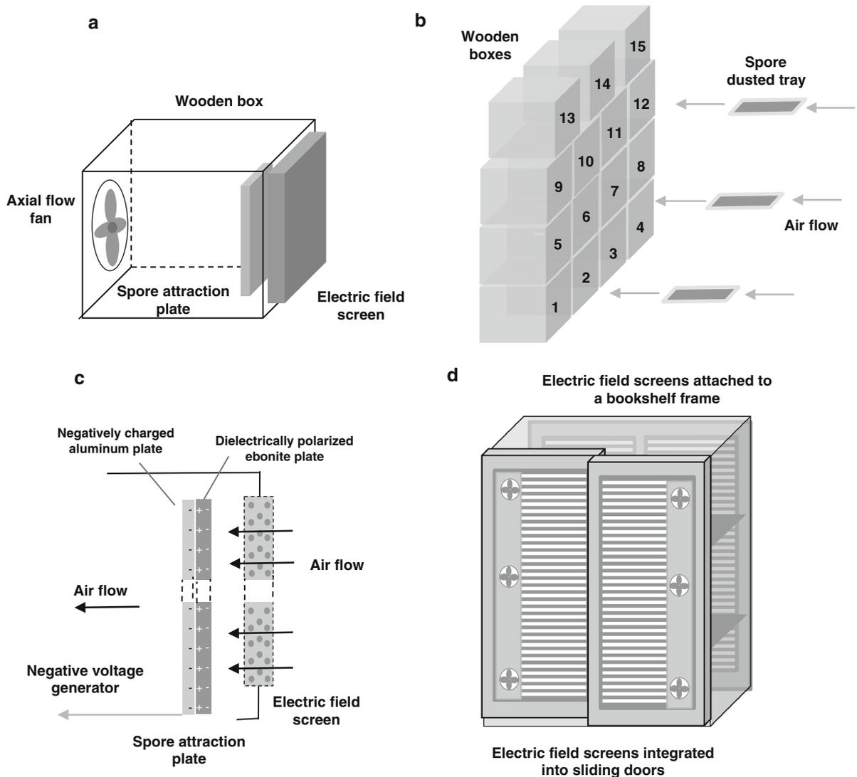
**Fig. 2** Diagram of screen-installed boxes (**a–c**) and bookshelf (**d**). **a** A test box furnished with an electric field screen and an axial-flow fan on opposite sides. **b** Positions of test boxes and the blowing of spores from parchment paper-covered trays towards electric field screens attached to the boxes. **c** A spore attraction
